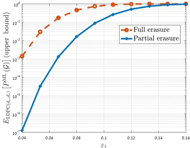
Fig. 6: A comparison of  $\mathbb{E}_{\text{LDPC}(d_v, d_c)} [P^{\text{ML}}(\mathcal{G})]$  for the LDPC ensemble  $(3, 27)$  (rate  $8/9$ ), for a GF(4) code of length 252. The set  $\{0, 1\}$  is either considered as a partial erasure or a full erasure with probability  $\varepsilon_1$ .
