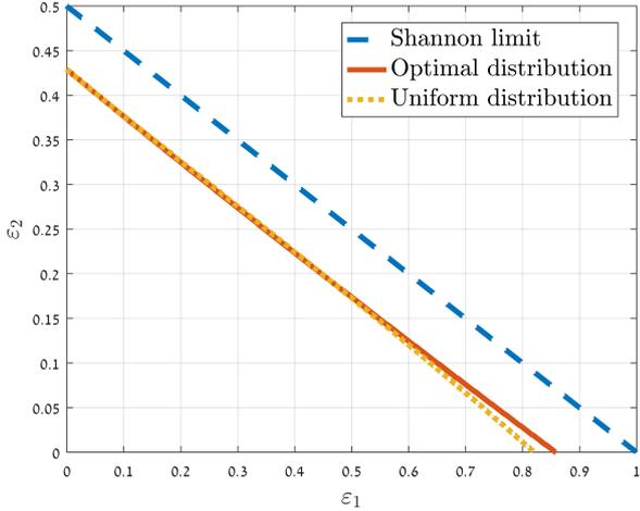
Fig. 2: The GF(4) QMBC  $\mathbb{L}$ -regions of two edge-label distributions for the (3,6) LDPC code ensemble. The QMBC Shannon capacity region is plotted for reference.
