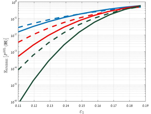
Fig. 4: Exact  $\mathbb{E}_{\text{SNBRE}} [P^{\text{ML}}(\mathbf{H})]$  as a function of  $\varepsilon_1$ , for  $\varepsilon_2 = \varepsilon_1/10$  and  $q = 4$  (solid lines). An asymptotically equivalent QEC with  $\varepsilon = (3/5)\varepsilon_1$  is also shown (dashed lines). The codeword lengths are  $n = 128, 256, 512$  (top to bottom) and the rate is  $8/9$  (Shannon limit: 0.185).
