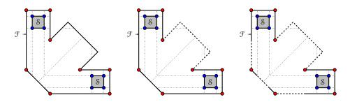
**Figure 12.** The solid lines represent the portion of the fence that needs to be considered, while the dashed lines represent portions that can be pruned and the thin dotted lines are the edges of the Voronoi diagram of *S* based on which the pruning is performed. (left) Original scenario, (middle) After pruning based on Lemma 7.1, (right) After pruning based on Lemmas 7.2 and 7.3.
