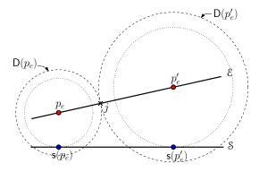
**Figure 7.** One step of the algorithm for disjoint segments, where  $\alpha > 1$ . The outer disks centered at  $p_e$  and  $p'_e$  are the critical disks of  $p_e$  and  $p'_e$ , and their radii are  $\alpha || \mathbf{s}(p_e) - p_e ||$  and  $\alpha || \mathbf{s}(p'_e) - p'_e ||$ , respectively. The algorithm places a jammer j at the intersection point of these disks.
