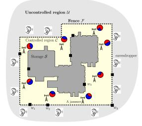
**Figure 2.** A "floorplan" of an example scenario, with storage S and the fence  $\mathcal{F}$  enclosing the controlled region  $\mathcal{C}$ . Jammers marked as antenna towers are placed between the fence and the storage.
