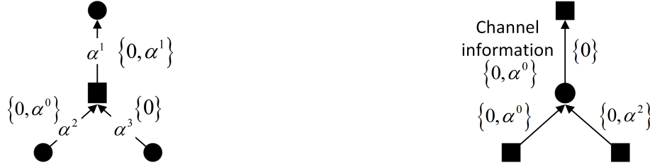
(a) An example for a CTV message over GF(4). The outgoing message is \frac{\alpha^2}{\alpha} \cdot \{0, \alpha^0\} + \frac{\alpha^3}{\alpha} \cdot \{0\} = \{0, \alpha^1\} .
