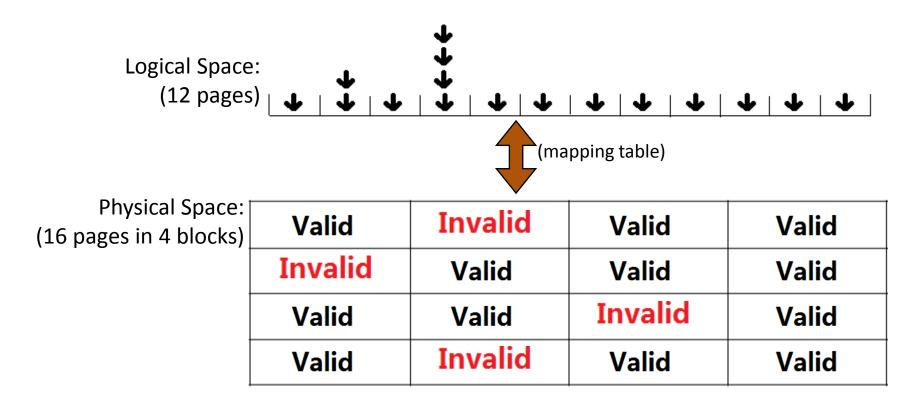
Initial condition: Start with an empty memory User writes uniformly and randomly distributed on user space stationary condition: Logical memory is always full (worst case)
