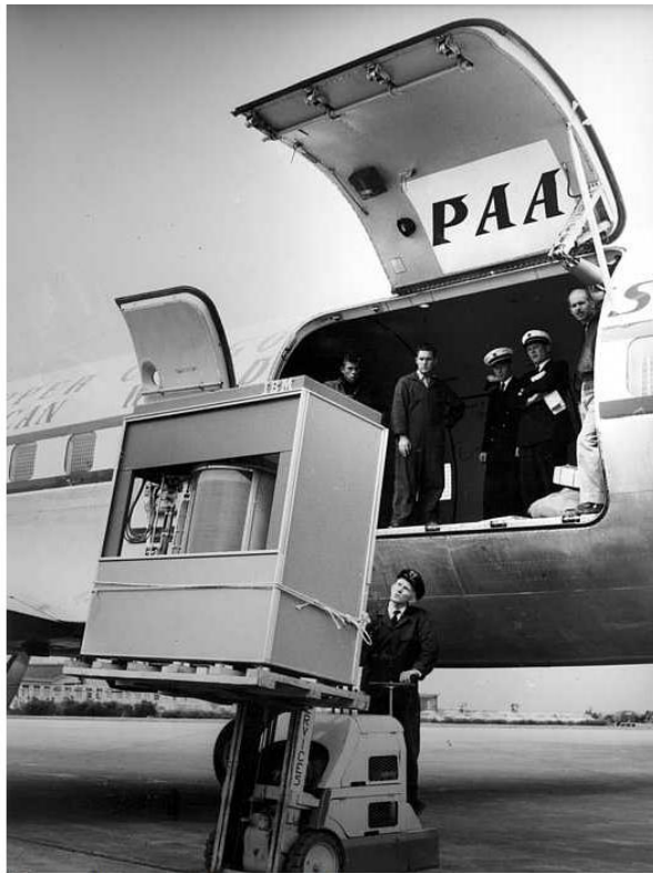
Above: An IBM Model 350 Disk File being delivered. Yes, that's ONE hard disk drive unit.
